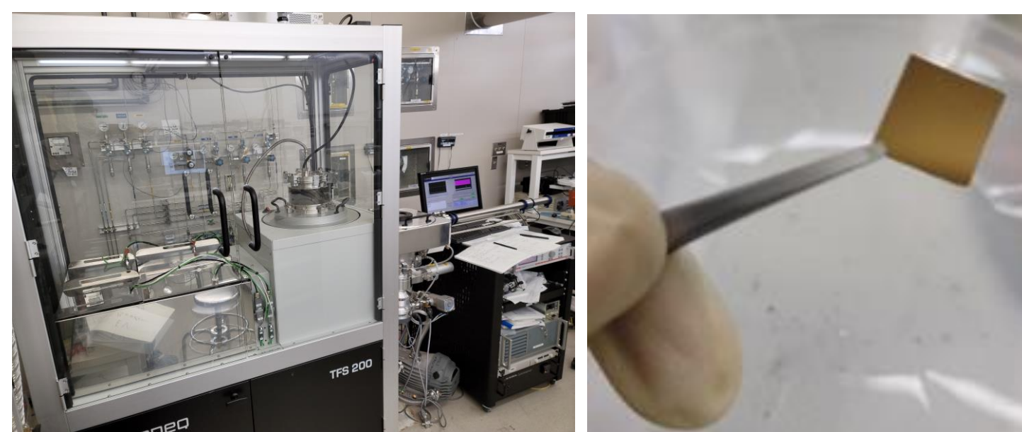
Figure 4. (a) Growth performed in Beneq TFS 200 plasma-enhanced ALD (PEALD) at MDL Cleanroom. \text{TiCl}_4 and Tetrakis(dimethylamido) titanium (TDMAT) precursors at 400^\circ\text{C} and 270^\circ\text{C} respectively. (b) \text{TiCl}_4 TiN films have good normal state R_{\square} = 0.85\Omega at 2490 cycles and \rho = 0.73\mu\Omega\text{cm} . TDMAT films have good R_{\square} = 4.7\Omega at 1250 cycles, and at comparable thickness, with R_{\square} = 5.6\Omega . Need to confirm the T_c [5].
