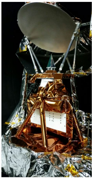
Fig.3. COWVR sensor in the thermal-vacuum chamber.
