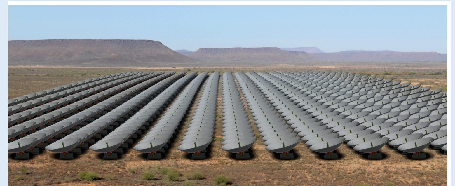
Fig 1: Rendering of HIRAX, a 1024 dish array to be built in the Karoo Desert, South Africa. HIRAX will operate between 400-800 MHz, with an associated redshift range of 0.8 < z < 2.5 , and is designed to constrain dark energy and its time dependence in over 1000 redshift bins by measuring the 100h^{-1}\text{Mpc} BAO scale as a function of time.
